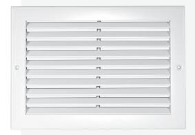
Models 5145H and 51FH Return Grilles have fixed horizontal blades (parallel to width/first specified dim.) spaced on 19mm centres with 45 $^{\circ}$  or 0 $^{\circ}$  straight face deflection.
